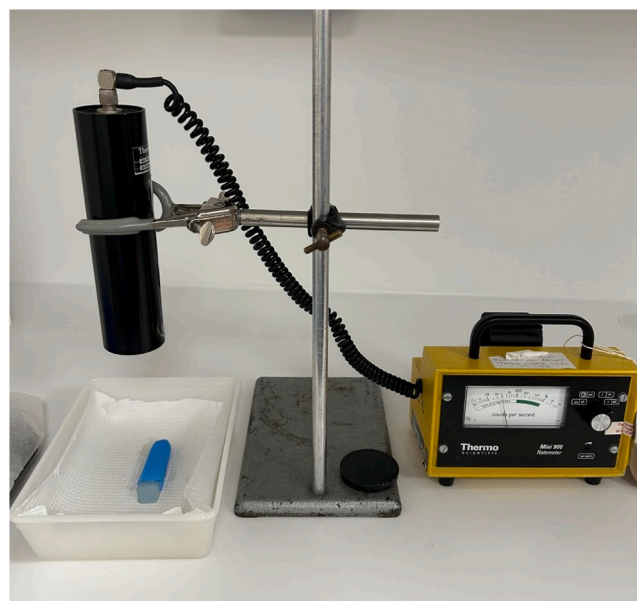
Fig. 1. Experimental set-up for activity measurements made with a Thermo Scientific Mini 900 contamination monitor.
